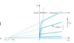
FIG 3. Early Effect—Finite Output Resistance
