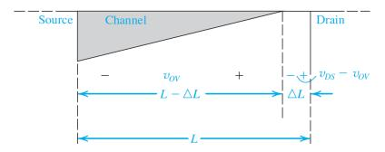
FIG 2. Early Effect—Finite Output Resistance
