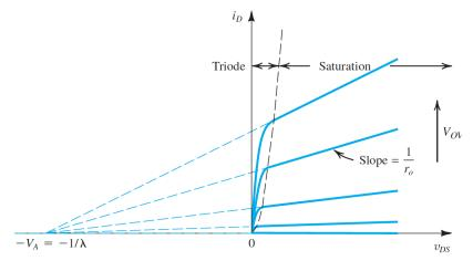
FIG 5. Early Effect—Finite Output Resistance
