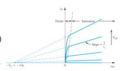
FIG 3. Early Effect—Finite Output Resistance
