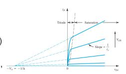
FIG 3. Early Effect—Finite Output Resistance
