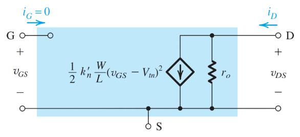
**FIG 4.** Large-Signal Equivalent Model of the n-channel MOSFET in saturation, incorporating the output resistance  $r_0$ . The output resistance models the linear dependence of  $i_D$  on  $v_{DS}$  and is given by Equation (4). Please note the addition of finite output resistance  $r_0$ .
